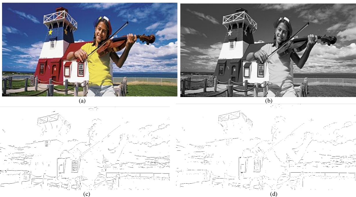
Fig. 2. Fuzzy edge detection method. (a) Color scale of an image, (b) Gray scale of an image, (c) Clear detected edges, and (d) Detected edges a bit unclear.
